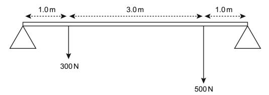
What are the upward forces from the two supports acting on the beam?
